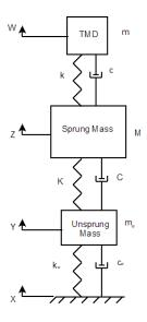
Figure 3: Quarter car model with TMD
