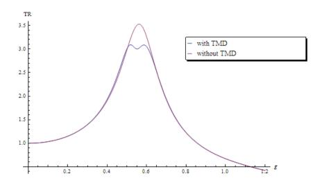
Figure 6: Half car transmissibility comparison
