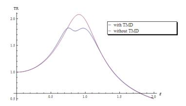
Figure 4: Quarter car transmissibility comparison
