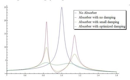
Figure 2: TMD comparison of systems with different damping
