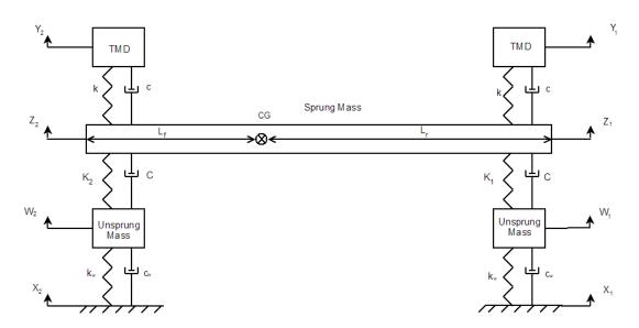
Figure 5: Half car model with TMD
